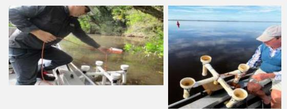
Figure 12: Sediment Accumulation Devises (Photo by Ecological Service Professionals)
